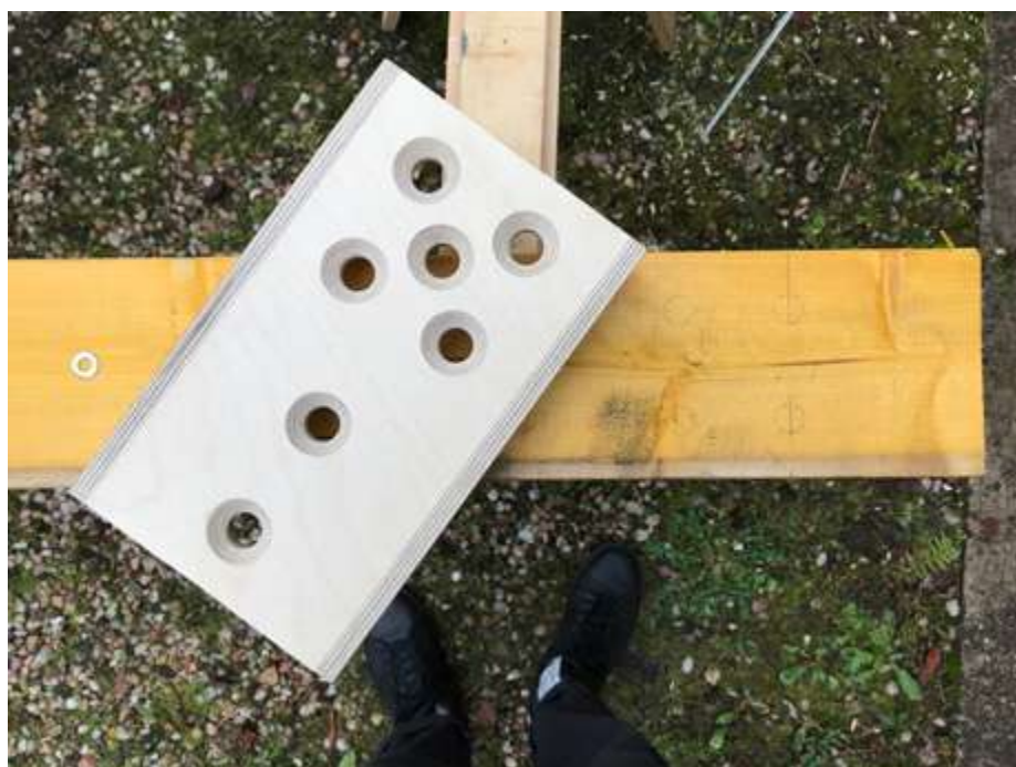
marking with a jig
