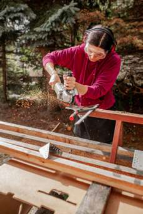
cutting metal with an angle grinder
