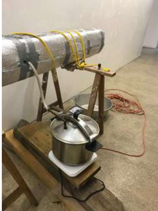
creating steam with a pressure cooker to bend the wood
